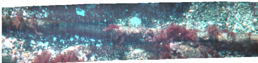
Fig. 1. Video mosaic of the coastal water of Costa Brava (Spain). Image alignment has been computed using an affine model with 6 DOF. Notice the large overlap (>90%) between consecutive frames.
