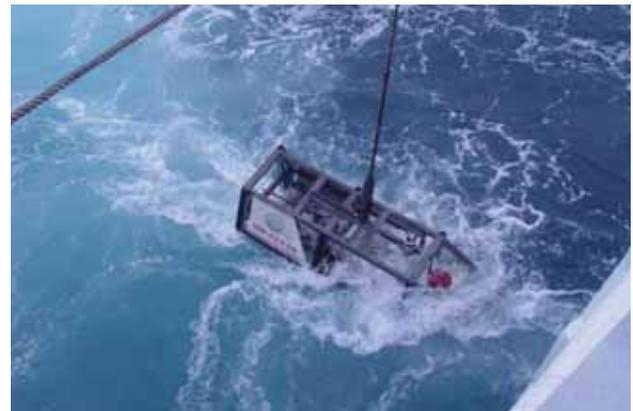
**Fig. 1.** The 6000-m integrated plume detection tow-system that was used during the DY115-19 expedition. This system includes video, camera, ADCP, CTD and USBL sensors, together with add-on MAPR and Mets sensors. Photo courtesy of DY115-19 Science Party.
