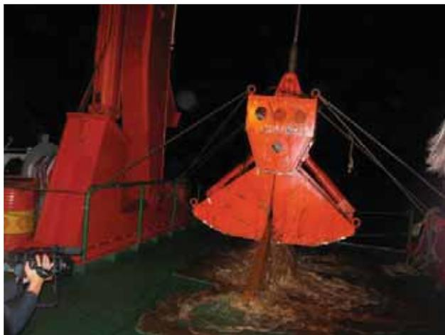
**Fig. 3.** TV-guided grab used during the DY115-19 expedition to recover hydrothermal sulfide deposits. The device was developed by the Pioneer Hi-Tech R&D Inc. in Beijing and funded by COMRA. Photo courtesy of DY115-19 Science Party.
