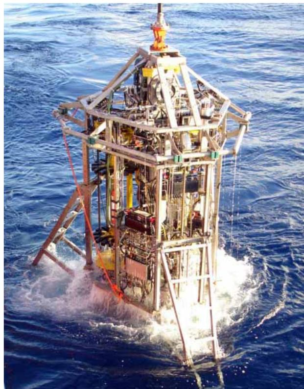
**Fig. 1.** The new Rockdrill2 is retrieved during cruise MSM03/2 of R/V *Maria S. Merian*.
