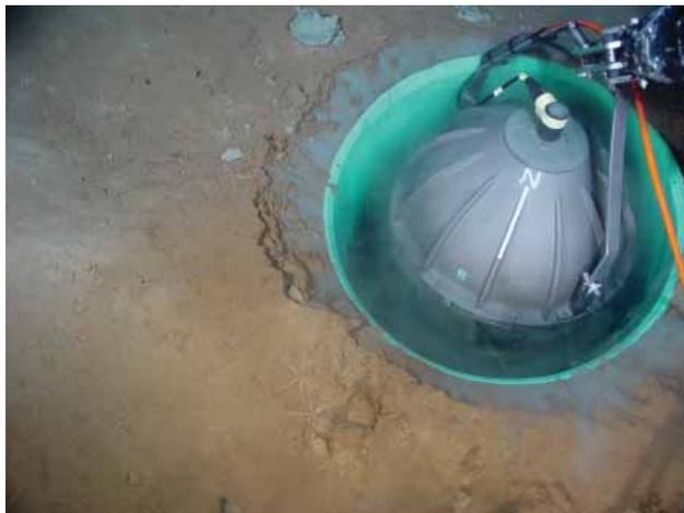
**Fig. 3.** Recovery of seafloor seismometer at Endeavour ISS. Image taken by ROV *ROPOS* during cruise led by University of Washington investigators that included initial work for NEPTUNE Canada.
