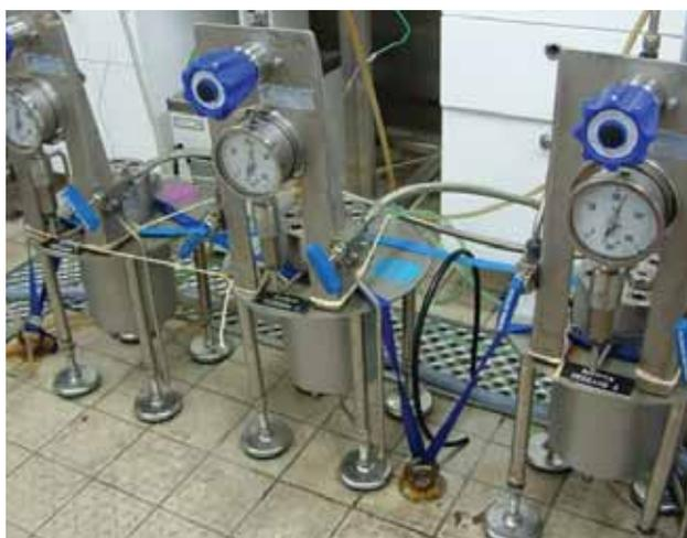
**Fig. 4.** The three pressure chambers of the DESEARES DEep-SEA RESpirometer (SB Roscoff).
