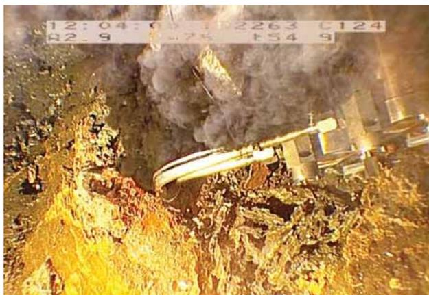
Fig. 3. Fluid sampling with titanium syringes.
