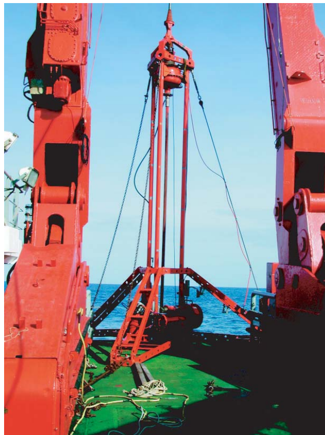
Figure 2. BGS Rockdrill during drilling operations with R/V Sonne in the New Ireland fore-arc and the Manus back-arc.
