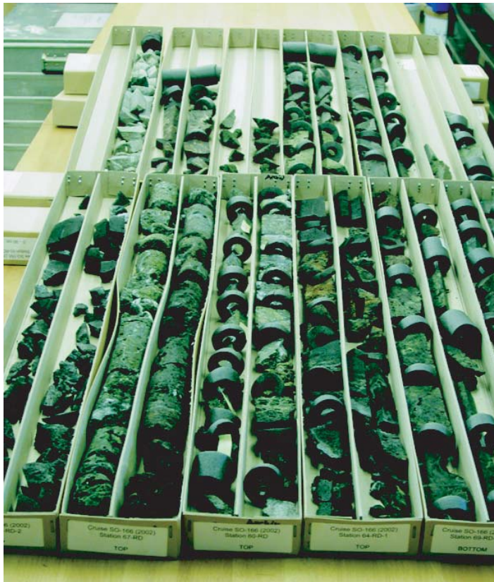
Figure 4. Drill core recovered with the BGS Rockdrill from the Manus hydrothermal field.
