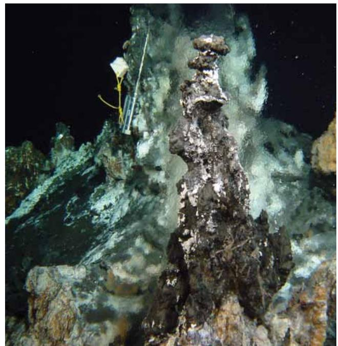
**Figure 1:** Autonomous temperature sensor installed at the White Castle Vent (Lucky Strike field). Bathyluck’09 Cruise (PIs J. Escartin and M. Cannat). Copyright: CNRS(INSU)/IFREMER.
