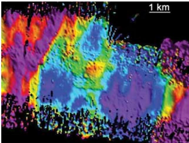
**Figure 2:** (left) A segment of raw Reson 8160 multibeam data (grid node spacing 50 m) showing a seamount and scarp (sampling targets on VSR2W). The multibeam swath echosounder was fitted to the hull of the R/V *Celtic Explorer* especially for the survey and achieved a swath width of ~3 km in 2000-m water depth.
