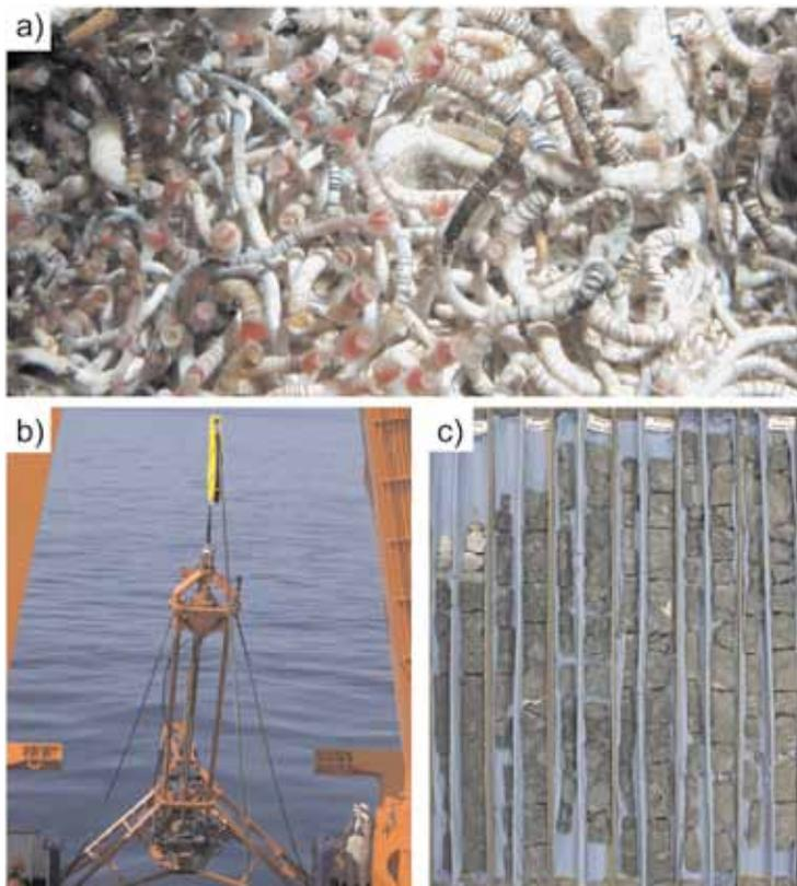
**Figure 3:** (a) Living siboglinid tube worms at the western summit of the Palinuro volcanic complex. (b) BGS Rockdrill 1 during operation onboard R/V *Meteor* cruise M73/2; (c) Drill core totalling 4.9 meters of massive sulfides and sulfates recovered from the Palinuro volcanic complex.
